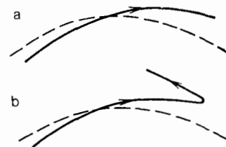
FIG. 1. Ray trajectories of (a) Alfvén wave and (b) an atmospheric whistler. The dashed lines are magnetic field lines.
