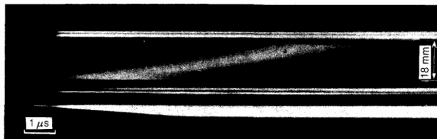
FIG. 13. Streak record of the motion of a bleaching wave in a solution of coumarin C6 in ether mixed with diphenylbutadiene in the absence of lasing (the pump source is shown below the cell).
