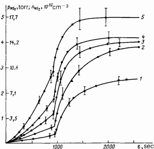
FIG. 2. Production of nitrogen oxide as a function of time for different starting air pressures (in Torr): 75 (1), 112.5 (2), 150 (3), 815 (4), and 300 (5) (the break in the curves occurs when the generator is switched off;  $t \approx 10^3 \text{ sec}$ ).
