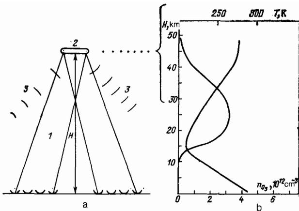
FIG. 1. Beams, plasma mirror (a), and distribution of the ozone concentration and temperature (b) (1: microwave beams, creating the plasma mirror 2; 3: relayed radiation).
