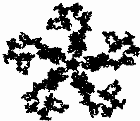
FIG. 11. The mapping point generates a diffusion fractal tree in the phase plane in the case of strong chaos, which preserves a q -fold symmetry. q = 5 , K_H = 20 , size of square 4 \cdot 10^3 \pi , time of 4 \cdot 10^4 mapping steps.
