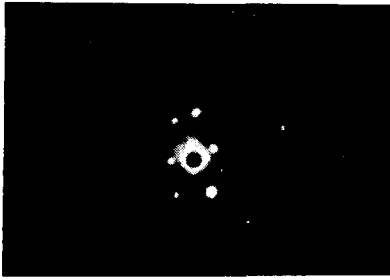
FIG. 16. Nanodiffraction pattern of a particle of bismuth molybdate 8 nm in diameter. 53
