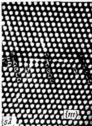
FIG. 35. Packing error of layers in the close cubic packing of gold atoms. 41
