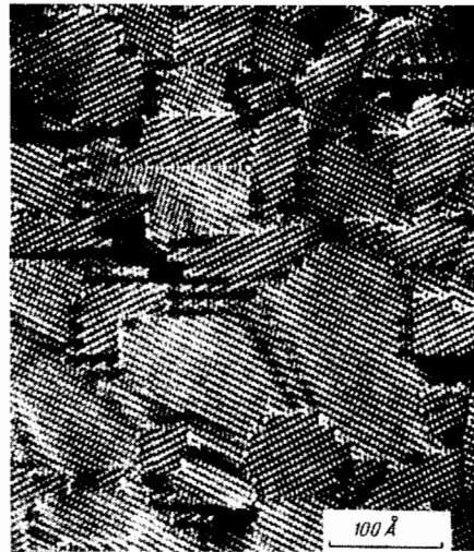
FIG. 44. A "carpet" of domains in the alloy Au, Mn 2 after annealing. 105 The domain boundaries often amount to twinning of the adjacent cubic packings.
