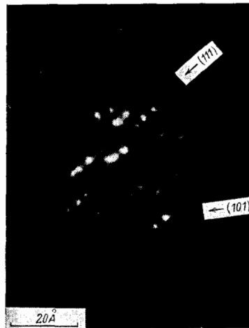
FIG. 3. Dark-field electron micrograph of a microcrystal of \text{ThO}_2 . 4 Bright spots are thorium atoms.
