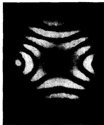
FIG. 14. Conoscopic pattern of a biaxial nematic. 80 KL (26%)–DeOH (6.24%)–H 2 O (67.76%) system. Thickness of specimen 2.5 mm. Temperature 20 °C.
