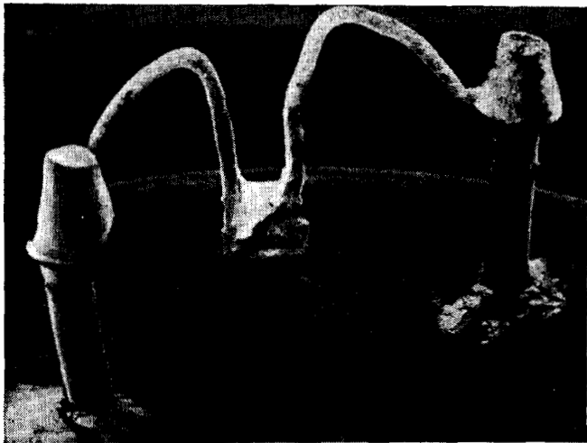
FIG. 2. One of the first gallium arsenide injection lasers (P. N. Lebedev Physics Institute of the Academy of Sciences of the USSR, 1962).
