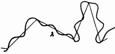
FIG. 4. Determination of the length of a curve with a scale length \lambda .
