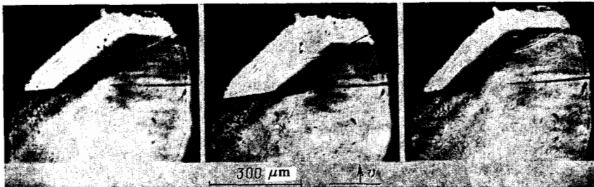
FIG. 28. Photographs of three consecutive positions of a kink on a domain wall in \text{YFeO}_3 at 110 °K, taken at 5-nsec intervals. 122 The time interval between two consecutive photographs is \sim 3 nsec.
