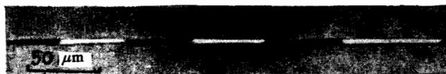
FIG. 1. 180° DW in an yttrium iron garnet plate, observed in polarized light with slightly uncrossed polarizers of the microscope. The Bloch lines separate the black and white subdomains in the DW.
