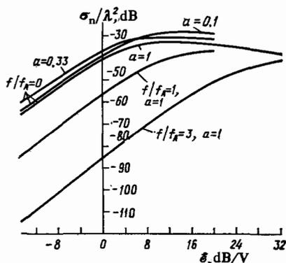
FIG. 6. Calculated dependence of the NESAs of a half-wave nonlinear vibrator on the amplitude of the emf induced in it. Parameters:  $a = R_A/R_0$ ,  $\beta = 1 \text{ V}^{-2}$ .
