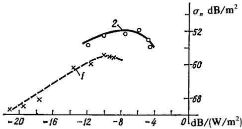
FIG. 7. Experimental dependence of the NES A of a half-wave nonlinear vibrator on the flux  $\Pi$  of the irradiating power. 1—vibrator with contact No. 1; 2—vibrator with contact No. 2.
