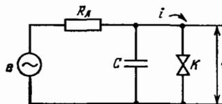
FIG. 4. Electrical circuit with a nonlinear contact.  $e(t)$  is the external emf,  $C$  is the capacitance of the contact,  $K$  is a nonlinear contact.
