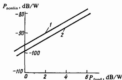
FIG. 2. Experimental dependence of the power  $P_{\text{nonlin}}$  of the IMI of the third order ( $f_c = 2f_1 - f_2$ ) on the power  $P_{\text{fund}}$  of the first harmonics for a contact in a coaxial line. The contact is formed by a sphere (radius 1.5 mm)-plane from polished aluminum. 1—pressure on the contact 50 g, 2—pressure on the contact 200 g.  $f_2 = 4156$  MHz,  $f_1 = 4021$  MHz,  $f_c = 3886$  MHz;  $P_{f_1} = P_{f_2} = P_{\text{fund}}$ .
