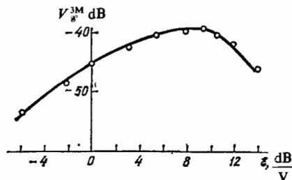
FIG. 3. Experimental dependence of the relative level of the third harmonic at the contact on the amplitude of the emf in the electrical circuit. The contact is made of steel (steel 20) in the form of a sphere (radius 3 mm)-plane, polished, and then oxidized in air at 400°C for 8 hours; the resistance of the external circuit is  $R_A = 200$  Ohm;  $R_0 = 100$  Ohm;  $\beta = 1.75$  V<sup>-2</sup>.
