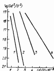
FIG. 1. Prebreakdown current flowing between clean parallel electrodes of tungsten, as a function of the voltage applied to the gap, plotted in the coordinates of the Fowler-Nordheim equation. 17 The interelectrode distance d has the following values in centimeters: (1)—0.005, (2)—0.0025, (3)—0.102, and (4)—0.406.
