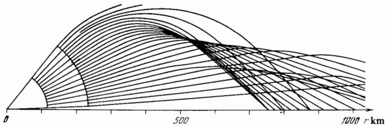
FIG. 2. Ray pattern when a ground-level point source of radio waves irradiates the ionosphere (from Ref. 1).
