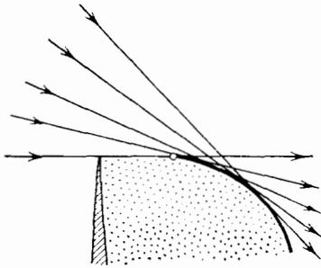
FIG. 23. Interrupted penumbral caustic which arises upon the screening of the primary wave in free space.
