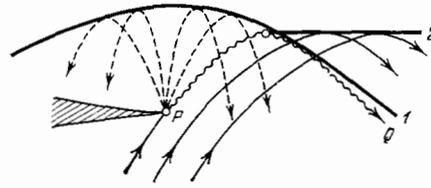
FIG. 24. Penumbral caustic 1 formed by diffraction waves (dashed curves) in a linear plasma slab. Boundary ray  $PQ$  touches both caustic 1 and the interrupted caustic 2, formed by ordinary rays.
