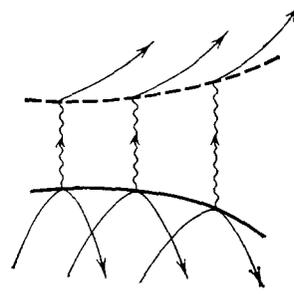
FIG. 25. Tunneling caustic. The lower branch (solid curve) corresponds to reflected rays, and the upper branch (dashed curve) corresponds to rays which tunnel under the barrier.
