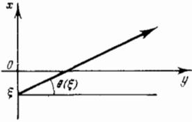
FIG. 6. Ray trajectory in the  $\{x, y\}$  plane in a homogeneous medium.
