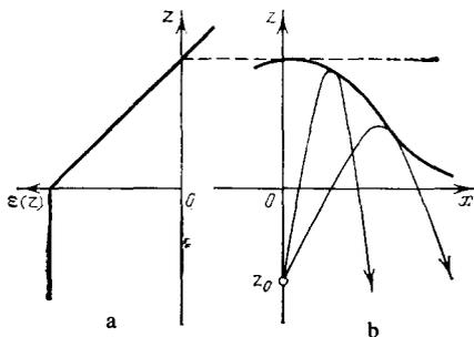
FIG. 16. a—Profile of the dielectric permittivity in the plasma slab; b—trajectories of rays describing the reflection of electromagnetic waves from this slab.
