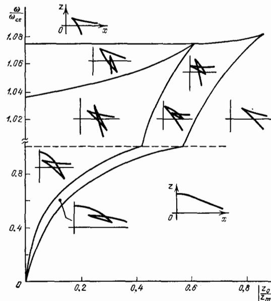
FIG. 20. Changes in the caustic pattern (two-dimensional sections of a butterfly) in the plane of the parameters  $\omega/\omega_{cr}$  and  $|z_0/z_m|$  for a parabolic slab with the dielectric permittivity profile from Subsection 2e.
