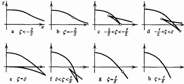
FIG. 18. Evolution of the shape of a caustic in a linear plasma slab.
