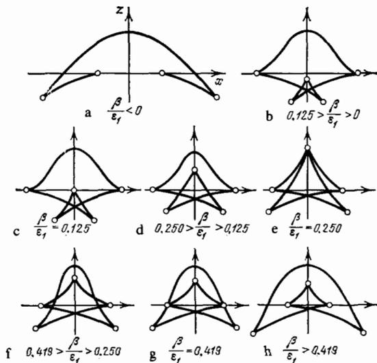
FIG. 21. Evolution of the shape of a caustic which arises in a linear plasma slab irradiated by a wave with a quadratic phase change in the  $z = 0$  plane.
