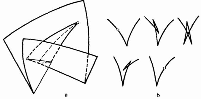
FIG. 15. Three-dimensional (a) and certain two-dimensional (b) sections through the caustic surface of type  $A_3$  (butterfly,  $m = 4$ ,  $l = 1$ ).
