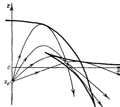
FIG. 17. Formation of a caustic loop (a projection of a swallowtail) upon the reflection of a spherical electromagnetic wave from a plasma slab with a linear profile of the dielectric permittivity.
