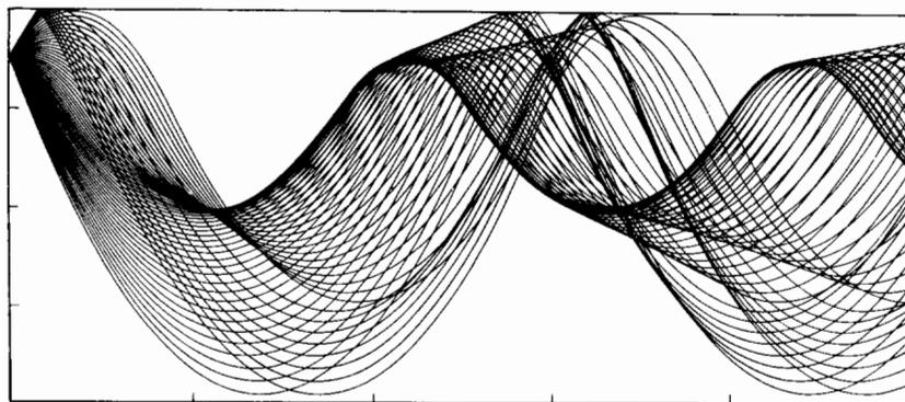
FIG. 3. An example of a ray pattern in an oceanic sound channel.<sup>3</sup>
