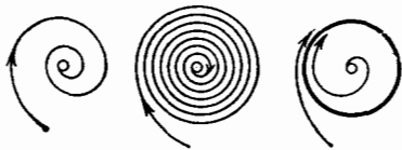
FIG. 23. Growth of a cycle when an equilibrium position experiences a soft loss of stability.
