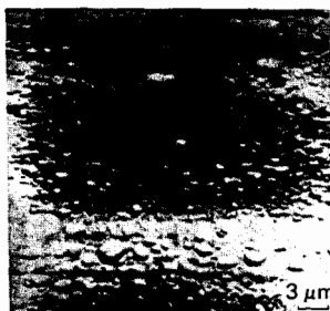
FIG. 20. Hydrogen blistering on an aluminum surface after implantation of 20-keV He + ions (dose D = 10^{18} cm -2 ) (Ref. 36).
