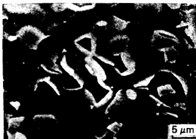
FIG. 7. Surface topography of type 0Kh16N15MZB stainless steel after bombardment with 40-keV \text{He}^+ ions ( 0.3T_m < T_{\text{bomb}} < 0.4T_m ). The bombardment dose is 10^{18} \text{ cm}^{-2} .
