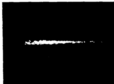
FIG. 22. Photograph of a laser spark in ordinary water.
