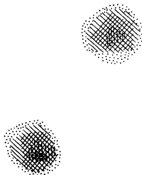
FIG. 4. NMR image of a cross-section of two parallel capillaries containing water. 5
