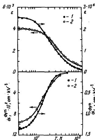
FIG. 1. Temperature curves of dielectric permittivity (left) and coefficient of dynamic nonlinearity (right) of strontium titanate and potassium tantalate crystals. 1—strontium titanate; 2—potassium tantalate.
