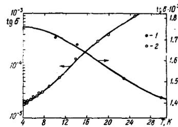
FIG. 2. Temperature dependence of dielectric loss tangents of strontium titanate (1) and potassium tantalate (2) crystals at 10 GHz.
