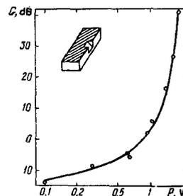
FIG. 3. Power gain vs pump power for parametric amplifier using strontium titanate crystal resonator.
