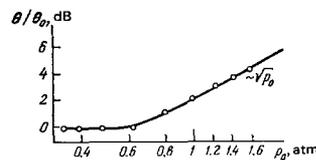
FIG. 4. Dependence of the relative width of the directivity characteristic on the amplitude of primary radiation.<sup>26</sup>
