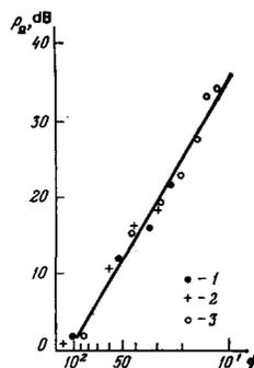
FIG. 6. Dependence of the level of the secondary radiation on the frequency reduction. 1—according to Ref. 31 at frequency of 105 kHz, 2—according to Ref. 31 at frequency of 123 kHz, 3—according to Ref. 29.
