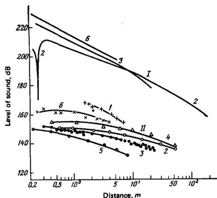
FIG. 5. Levels of the Primary (I) and secondary (II) radiations at the axis as a function of the distance. 1—according to Ref. 27, 2—Ref. 7, 3—Ref. 29, 4—Ref. 24, 5—Ref. 23, 6—Ref. 30.
