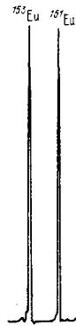
FIG. 4. Mass spectrogram showing the emergence of either the isotope 153 Eu (at the left) or 151 Eu (at the right) as the wavelength of the exciting laser is tuned. 16
