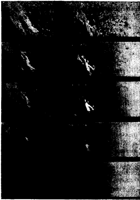
FIG. 15. Magnetograms of two regions on the solar disk obtained on the Kitt Peak Observatory magnetograph in the range 2–2000 \Gamma . All 4 prints (top) were taken from the same magnetogram with the image reproduced at various gains—1:2:4:16. The photographs at the bottom are of the same regions in visible light.
