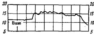
FIG. 4. Profilogram of erosion track left by a spot of the second type on a copper cathode.
