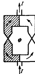
FIG. 12. Thermoelectric circuit containing two Josephson barriers (quantum interferometer). The flux in the ring is \Phi = \Phi_T + \Phi_e , where \Phi_e is the external flux.
