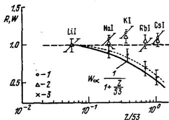
FIG. 8. Formation of the  $\pi$ -mesic atom of iodine as a function of the atomic number  $Z$  of the alkali metal bonded to it.<sup>[27]</sup> 1, 2—experimental ratios of  $\gamma$ -ray photopeaks due to the products of nuclear absorption of pions in iodine and in a monitoring material; 3—probability of formation of the  $\pi\text{I}$  atom. Solid line—Fermi-Teller Z-law. All numbers normalized to LiI.
