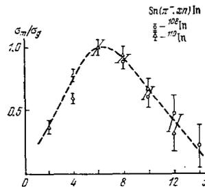
FIG. 7. Dependence of the isomeric ratio in the  $\text{Sn}(\pi^-, xn)^{108,110}\text{In}$  reaction on neutron multiplicity. Normalized to the case  $x = 6$ .
