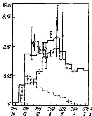
FIG. 3. Neutron multiplicity in the  $^{208}\text{Pb}(\pi^-, xn)^{208-x}\text{Tl}$  reaction. Dashed line—calculations based on the quasideuteron absorption mechanism, dot-dash line— $\alpha$ -particle mechanism, solid line—obtained on the assumption that 25% of all events involve pion absorption by an  $\alpha$ -cluster and 75% by a quasideuteron. Level density parameter  $a = 0.1 \text{ MeV}^{-1}$  (figure taken from paper by Il'inov *et al.* [20]).
