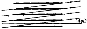
FIG. 23. Soller collimator limiting the divergence of recorded radiation in the vertical plane.
