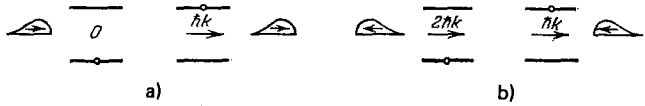
FIG. 6. Acceleration by a \pi -pulse of an atom in the ground state (a); acceleration of an excited atom by a \pi -pulse running in the opposite direction (b).
