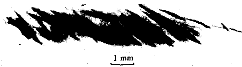
FIG. 11. X-ray topogram of quartz crystal. The spatial resolution is better than 1 micron; edge dislocations are visible.
