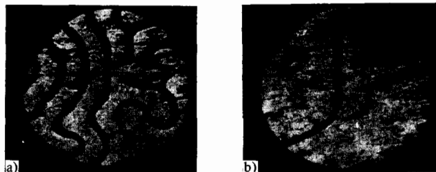
FIG. 6. Domain structure of orthoferrite: a) without magnetic field; b) in the field of a permanent magnet.
