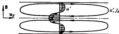
FIG. 3. Schematic illustration of additional motion and Hall currents during the development of overheating-convective instability.
