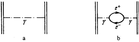
FIG. 4. Electromagnetic interaction of two heavy particles (a) in lowest order in the coupling constant and (b) with allowance for the screening of the initial charges by a virtual electron-positron pair. [In the figure the dashed-dotted line denotes a "Coulomb" photon.]
