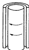
FIG. 4. Generator that can be easily realized in experiment. The inner cylinder, of radius r_0 , rotates; a gap \Delta r exists between the inner and outer cylinders.
