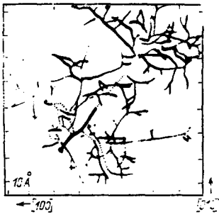
FIG. 4. Projection on the (001) plane of the trajectories of the atoms ejected from their sites in a cascade of collisions in \alpha -Fe. [2] This cascade was initiated by a primary knock-on atom of energy 5 keV that left its site at the lower end of the heavy solid line. The dots are the tracks of the secondary knock-on atoms. The solid thin lines show the trajectories of the knock-on atoms of higher orders.
