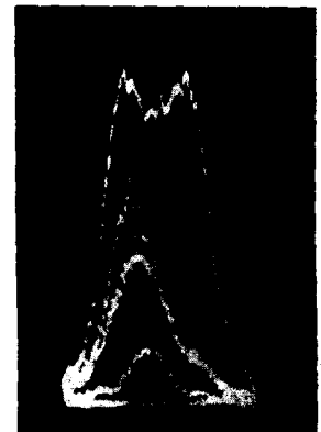
FIG. 3. Intensity distribution of the recombination radiation over the cross-section of an n-InSb specimen: [58] H (Oe) = 0 (1), H = 200 (2), 400 (3), and 1000 (4). The current I_p in the plasma = 50 A, and the current-pulse duration \tau_{\text{pulse}} = 4 \mu\text{sec} .
