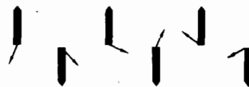
FIG. 4. Illustration of the disorder in orientation of nuclear moments (small arrows) in a crystal with ordered atomic moments (heavy arrows).
