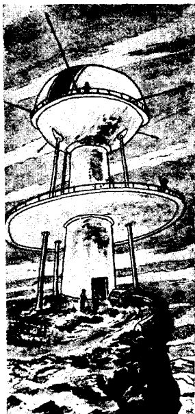
FIG. 8. Artist's conception of the general appearance of the tower of a ground-based telescope matched thermally and aerodynamically with the free atmosphere. In construction of such a tower it is necessary to make aerodynamical studies which make it possible to avoid the cold air near the earth being thrown to the height of the instrument and to avoid the appearance of cold air near the radiation-cooled parts of the tower, cupola, and telescope.
