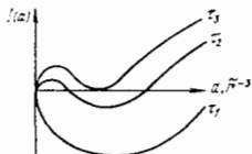
FIG. 6. Typical plots of I vs a (or \tilde{r}^{-3} ) in solutions or in paramagnets in the critical region at different relative temperatures \tau_1 = 0 < \tau_2 < \tau_3 = \tau^* .
