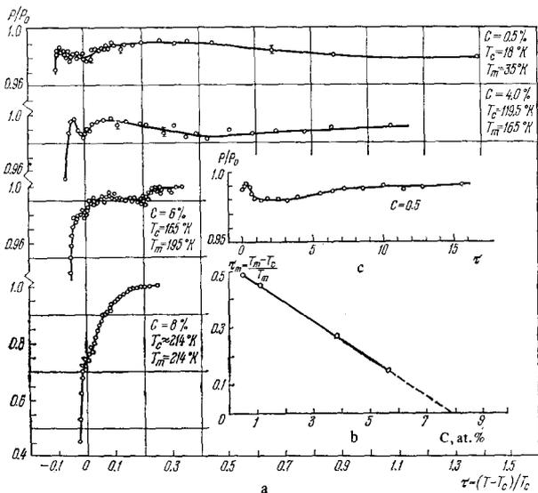
FIG. 2. Temperature dependence of the polarization of a neutron beam passed through a Pd-Fe sample with Fe concentrations from 0.5 at. % (a, c) to 8 at. % (a), and the shift of the high-temperature depolarization anomaly  $\tau_m$  to  $\tau = 0$  (b).
