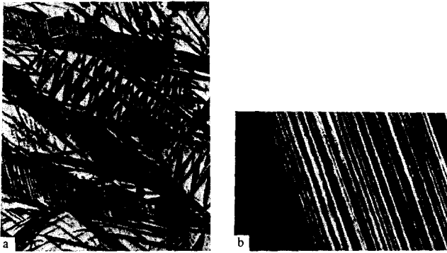
FIG. 1. Macro- and microstructure of the alloy Fe-33% Ni after a martensitic transformation (X500 (a) and X10,000 (b)).
