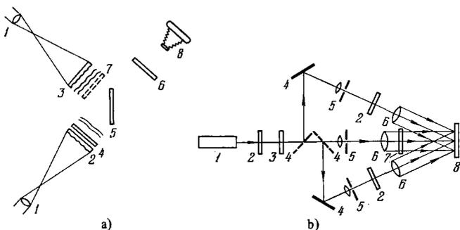
FIG. 2. Holographic schemes in which false polarization states can be eliminated by using: a) a depolarizing diffuser (1—micro-objectives, 2—scatterer, 3—diffuser; 4—object, 5—photographic plate, 6—analyzer, 7—polarizer, 8—photographic camera); b) thick emulsions (1—HeNe laser, 2—polarizers, 3— $\lambda/4$  plate, 4—mirrors, 5—micro-objectives with pinhole diaphragms, 6—lens systems, 7—object, 8—hologram).
