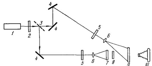
FIG. 3. Experimental setup for visual observation of polarization contrast. 1—He-Ne laser; 2— $\lambda/4$  plate; 3—semitransparent mirrors; 4—100% mirrors; 5—polarizers; 6—micro-objectives; 7—scatterer; 8—object; 9—photographic plate; 10—photographic camera.
