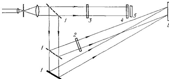
FIG. 1. Schematic diagram of setup for holographic recording and reconstruction of the vector characteristics of a field. 1—Mirrors; 2— $\lambda/2$  plate; 3— $\lambda/4$  plate; 4—scatterer; 5—object; 6—hologram.
