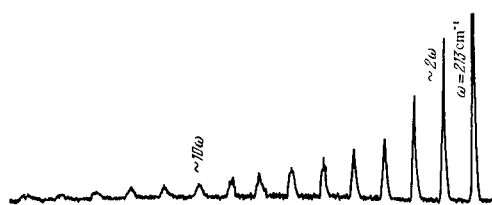
FIG. 5. Resonance RS spectrum of iodine vapor excited in the continuum region of the ^1\Sigma_g^+ \rightarrow ^3\Pi_{0u} band ( \nu = 20,487 \text{ cm}^{-1} ) [121a].
