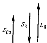
FIG. 1. Diagram showing the orientation of the spin and orbital moments in alloys of RCo_5 .
