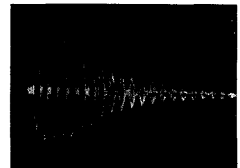
FIG. 3. Series of second-harmonic pulses (10 MHz) in magnesium-aluminum alloy. Voltage of 5 MHz radiator is 1000 V (maximum). Rod length 7.5 cm.
