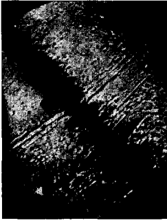
FIG. 5. Image of working surface of a magnetic recorder head in an emission microscope with an aperture diaphragm, with the magnetizing current flowing through the winding of the head [76]. The figure shows the gap region in the form of a dark band.
