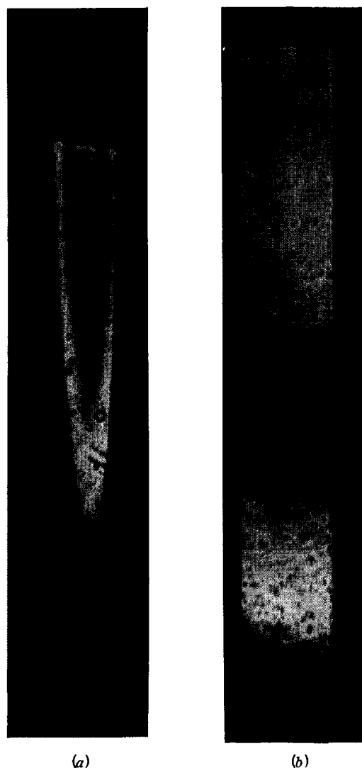
FIG. 2. (a) Interference of the elastic twinning lobe in a calcite crystal. (b) Interference produced in an elastic twin in calcite by knife-edge loading.
