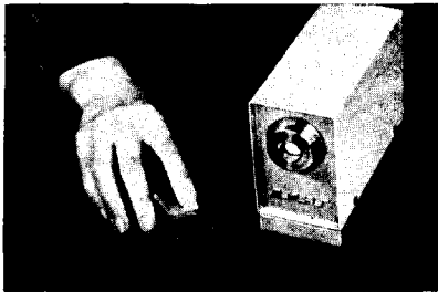
FIG. 3. Portable x-ray pulsed nanosecond generator RING. Operating voltage 150 kV; weight 1.4 kg.
