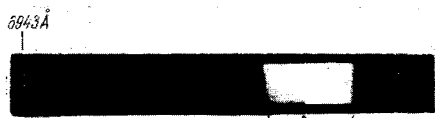
FIG. 17. Stimulated Raman spectrum of a cryptocyanine solution obtained at maximum laser power and at a concentration of 0.5 \times 10^{-4} moles/liter. The brackets indicate the different laser-action bands.
