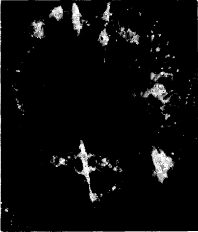
FIG. 9. Helium ion image of a tungsten tip ( T = 78^\circ\text{K} ). Neutron irradiation led to the formation of a large dispersed cluster. [39]
