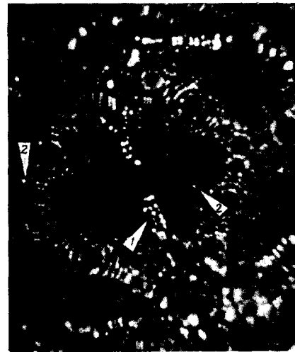
FIG. 3. Helium ion image of a tungsten tip ( T = 78^\circ\text{K} ). [20] The arrows indicate atoms which have been displaced by the forces of the electric field into metastable positions.
