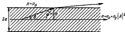
FIG. 1. Illustration of the derivation of a formula for the critical power of a beam, transported without divergence (self-trapping) in a nonlinear medium. The shaded area is occupied by the beam.
