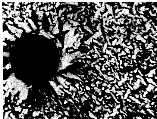
FIG. 1. The liquid-crystalline phase of cholesteryl benzoate between crossed Nicols of a polarizing microscope. Dark circle—air bubble. Magnification 540 \times .
