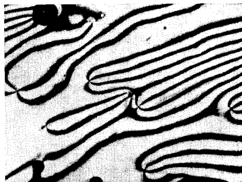
FIG. 8. Nuclei and dark branches proceeding from them. Liquid-crystalline texture of p -azoxyanisole. Magnification 120 \times .
