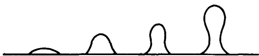
FIG. 10. Variation in the shape of the vapor bubbles on a horizontal surface with increasing bubble volume.
